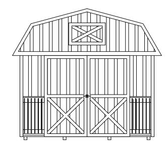
NOTE: ATTACH PORCH GUARD RAIL WITH (2) #8 X 2½" SCREWS AT EACH UPRIGHT
