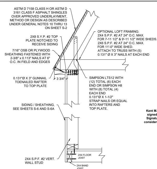
TOP PLATE TO RAFTER AND FLOOR FASTENING DETAIL
